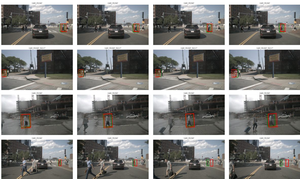
Figure 3: Qualitative results on NuScenes dataset. From left to right, all predictions are depicted. The green is the ground truth and the red is the predicted bounding box.
