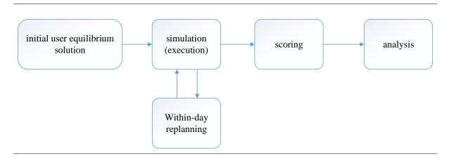
Figure 3: The Agent-based simulation approach (within-day replanning)
