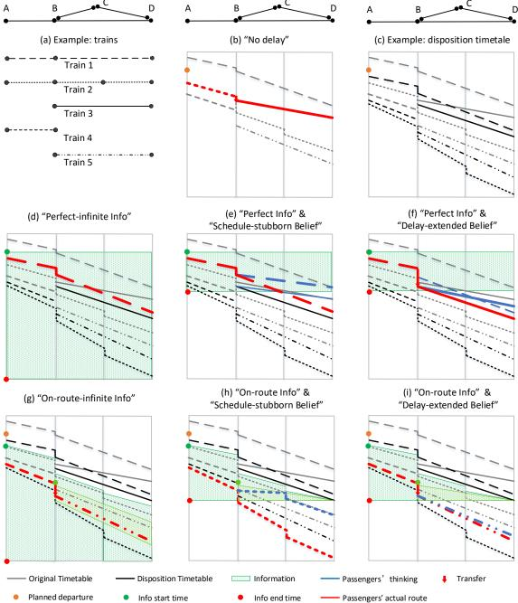
Figure 1: Explanation of incomplete information and passengers' belief
