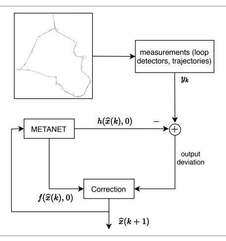
Figure 1: The flowchart of the proposed framework.
