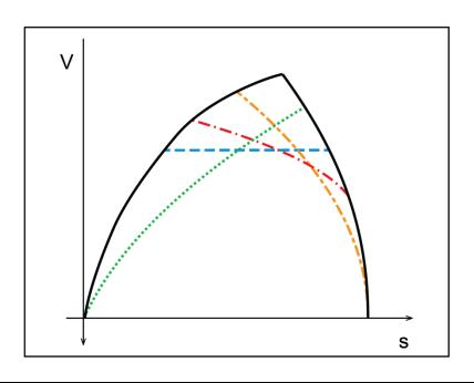
The black line represents the minimal running time for a given case. This strategy illustrates the maximum energy consumption<sup>2</sup>. The different colours represent different strategies, how to reduce the maximum energy consumption:
