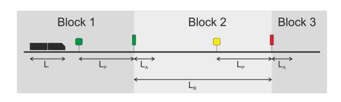
L is the length of the train.  $L_B$  is length of the section block.  $L_P$  is the distance between the advance signal and the main signal.  $L_A$  is the overlap.
