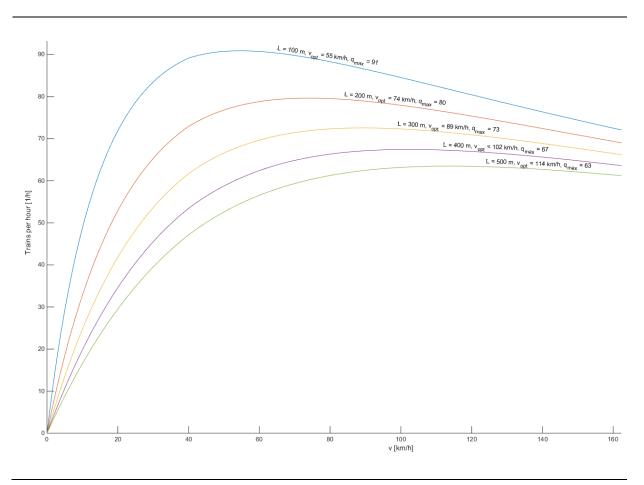
Figure 6 Maximum line capacity for automated trains
