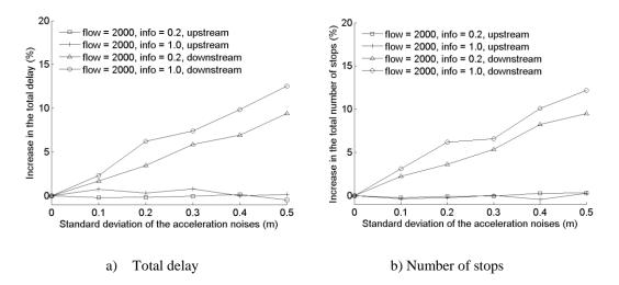
Figure 3. The robustness to the acceleration errors.
