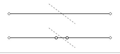
Figure 3: The crossings XML input file lists every link that crosses a public transport link (rail tracks in most cases). Usually the crossing links are the same for opposite public transport links. The order of the crossing links is irrelevant, the file is only used to connect the public transport links and their crossing links.
