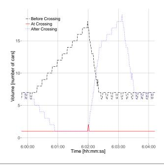
Figure 7: This Time-Space Diagram illustrates on the simplistic scenario how the cars are "queueing" in front of the closed crossing. Actually their travel-times are adapted in order to arrive at the crossing when it reopens. The plot only takes into account the *linkLeaveEvents*, since one cannot track an individual vehicle on a link.
