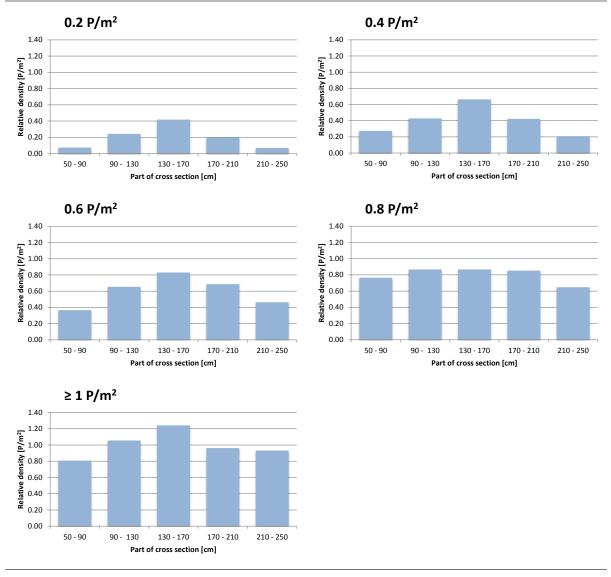
Figure 5: Densities measured outside the lecture hall at ETH Zurich. Shown are relative pedestrian densities of cross section segments, for different macroscopic flow densities.
