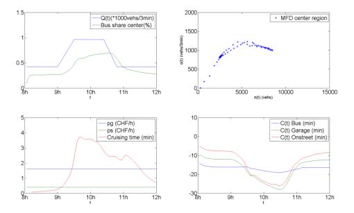
Figure 2 System dynamics and traffic performance under fix parking pricing scheme: (top left) mode share of bus and total travel demand over time, (top right) the MFD of the center region with congestion observed, (down left) the prices of  $p_s$  and  $p_g$ , and cruising-for-parking time, and (down right) the total cost of each mode  $C_k$  over time.
