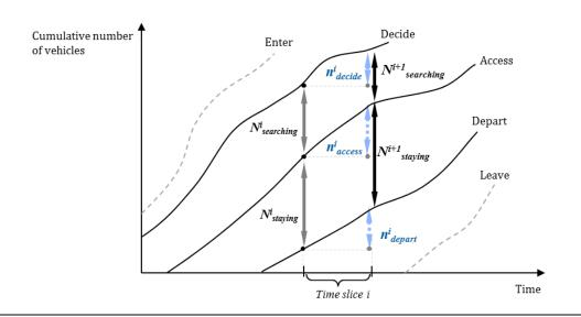
Note that the dotted line in Figure 2, "enter" and "leave" indicate the cars which enter and leave the area. The number of vehicles going through these two events are obtained based on assumptions on travel demand (i.e., input to the model). For a time slice (e.g., one minute), each state of the system can be updated based on:
