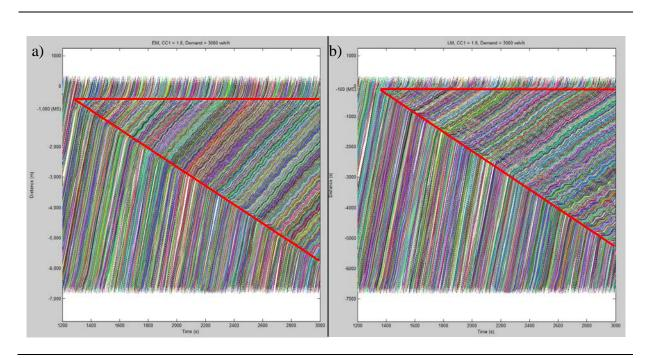
Figure 6 Time-space diagram using Parameter Set 4 (CC1 = 1.8), demand = 3,000 veh/h
