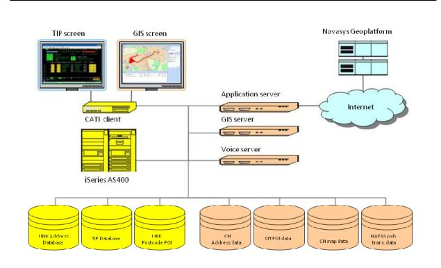
Fig. 1 Hardware and software concept for the MCMT 2010
