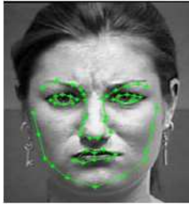
Figure 4: Mask tracked by AAM along a video sequence
