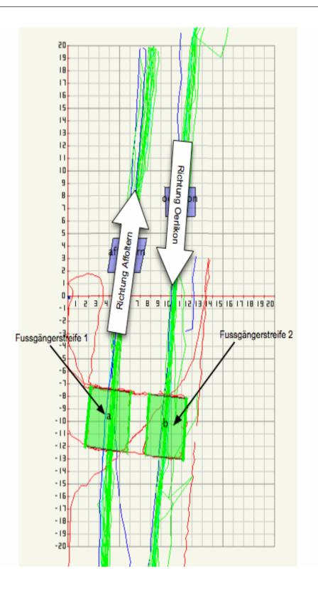
The illustration shows the installation of the laser-sensor at a pedestrian-crossing (green rectangles) The cars are green lines, the bicycles are blue lines, and the trucks (or buses) are light blue. The red line shows the pedestrian who was marking the site of the pedestrian crossing with central island.
