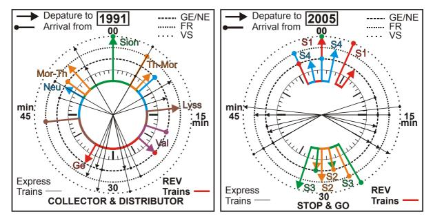
It is obvious that the first goal of the new REV system is to be a true rapid-transit rail system. Two minutes is the most usual stop time for REV trains at Lausanne. Connections between REV trains and Express trains are granted, but the waiting time is about a quarter of an hour. Such a waiting time may be considered as relatively high, even in the case of Lausanne, which is an important railway node [6].
