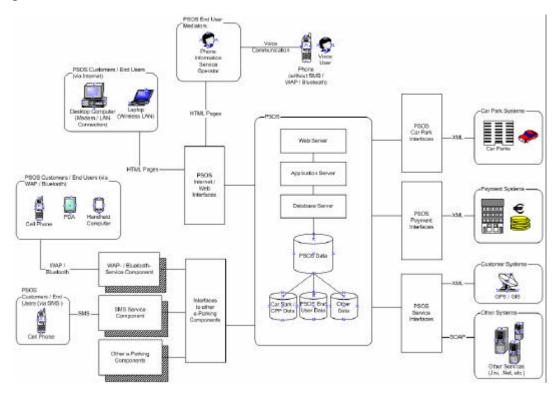
Figure 4: Software architecture
