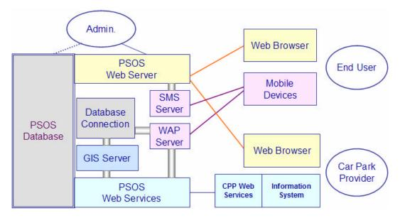
Figure 7: PSOS Block Diagram
