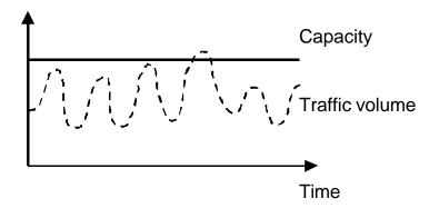
The capacity of roads are determined by measurements of traffic volumes. In contrast to other engineering sciences the system does not break as a result of the load itself. There are also some random effects which influence the breakdown probability. In addition to that even the capacity could not be compared with some kind of constant resistance. E. g. light and weather circumstances are significant effects.
